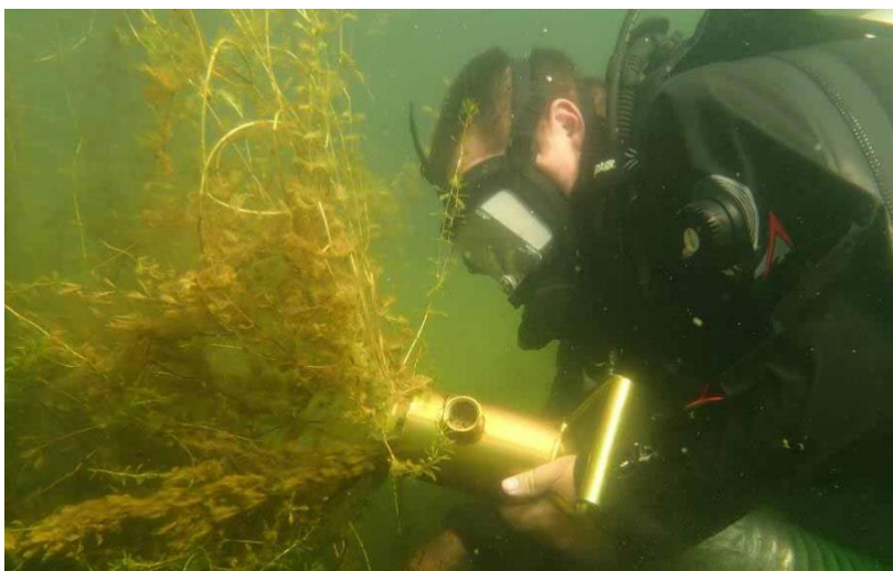
Figure 66: DASH - Diver Aided Suction Harvest (Chuck Druckery, 2016 Wisconsin Lakes Convention Presentation)
