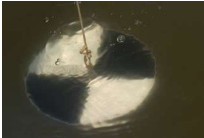
Figure 8 – Black and White Secchi Disk for measuring Water Clarity
