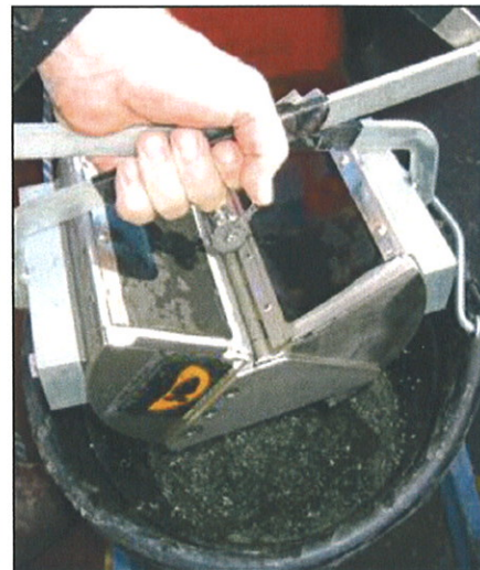
Figure 6. Photograph of petite Ponar sampler, sifting bucket, and sediment sample.
